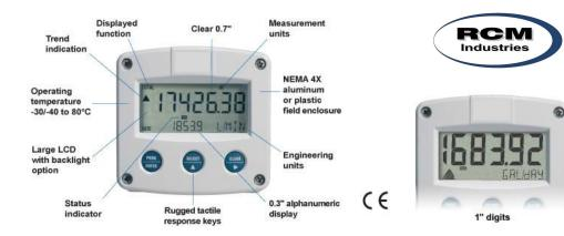
**New** Digital display flow meter 2 wire loop powered 4-20mA DC transmitter features 7 digits for flow rate and 11 digits for accumulated total. On-screen engineering units are easily configured, while different units for flow rate and total can be displayed simultaneously. A wide selection of options further enhances this models capability. Optional backlighting is available for easy viewing and intrinsic safe approval for hazardous locations.
